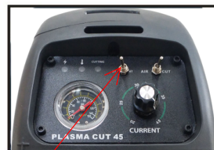
(5) select 2T or 4T torch control .2T is standard manual operation mode (6) Set the amperage dial and ensure switch is in Cutting mode
