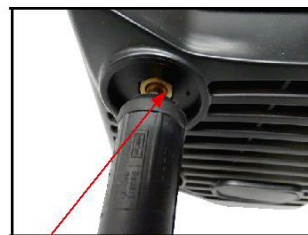
(2) Connect the earth lead to the output terminal of the machine and tighten.
