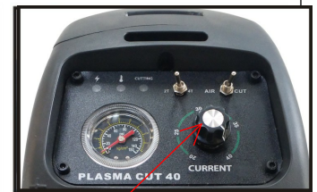
(5) select 2T or 4T torch control .2T is standard manual operation mode (6) Set the amperage dial and ensure switch is in Cutting mode
