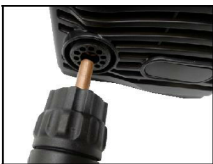
(1) Connect the Plasma Torch to the machine. Insert the torch connection into the torch connection receptacle at the front of the machine and screw up hand tight. Caution: Do not to bend the pins located inside the torch connector.
