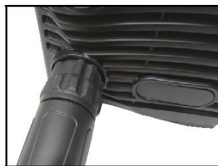
(1) Connect the Plasma Torch to the machine. Insert the torch connection into the torch connection receptacle at the front of the machine and screw up hand tight. Caution: Do not to bend the pins located inside the torch connector.
